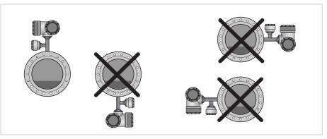
Figure 3-10: Mounting position
