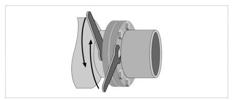
Figure 3-11: Tightening of bolts
