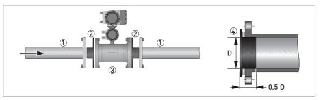
Figure 4-1: Grounding with grounding rings
