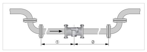
Figure 3-3: Recommended inlet and outlet sections, top view (1)  $\geq 5$  DN (2)  $\geq 3$  DN
