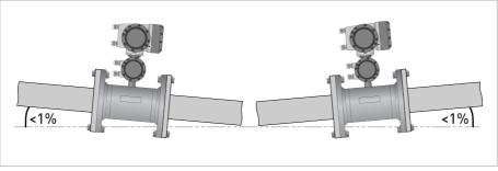
Figure 3-5: Recommended slope
