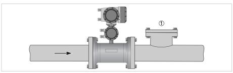
Figure 3-8: Option for cleaning of flow sensor
