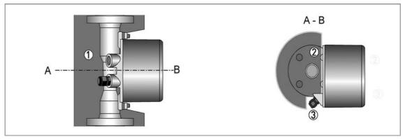
Figure 3-1: Insulation - cross section
