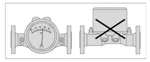
In order to comply with thermal parameters and measuring accuracy, H250H flowmeters for horizontal installation are to be installed in the pipeline so that the display is located on the side of the measuring tube. The maximum product and ambient temperatures indicated as well as the measuring accuracy are based on lateral installation of the display.
