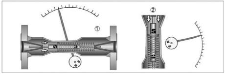
Figure 1-1: Operating principle H250H and H250U
