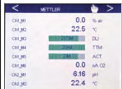
A configurable display allows the highest flexibility to view the most important values. The Wizard set-up allows the definition of favorites to directly reach any menu.
