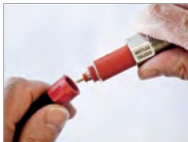
Plug and Measure feature offers pre-calibration of sensors and, in combination with the auto-recognition function, greatly simplifies sensor handling.
