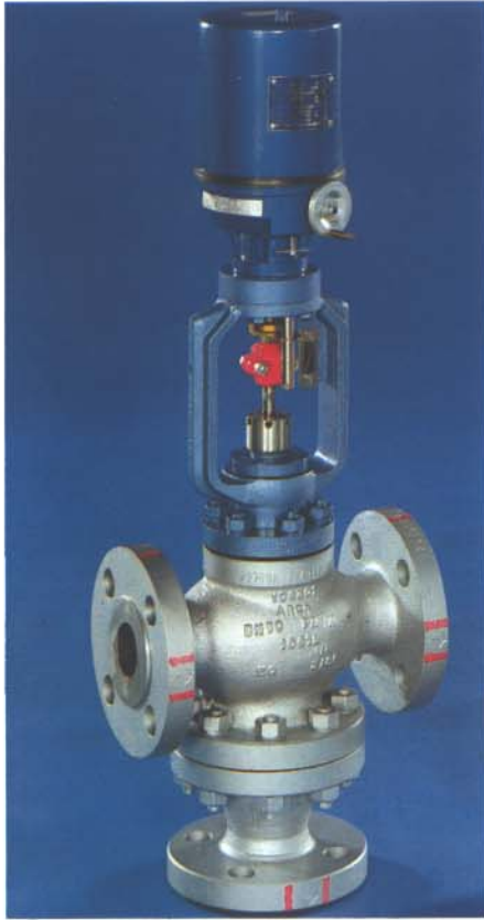
Pressure control- and mixing valve for hot water in a teleheating station DN 50, PN 100, with electric actuator series 853.
